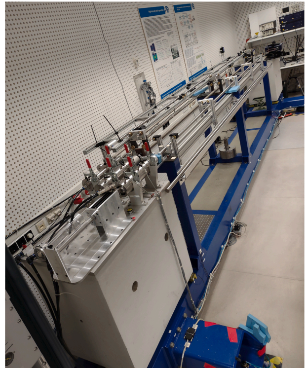
Fig. 7. Hopkinson bar shock generating device with linear motor and pneumatic actuators on the bottom left side.
