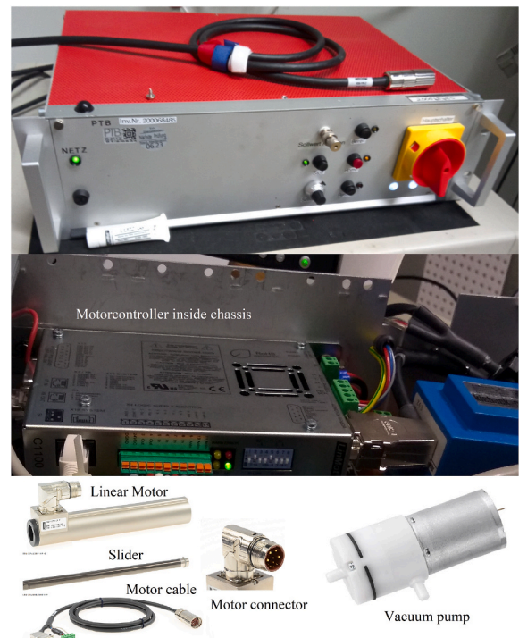
Fig. 10. Fig. 10: Control box (top), inside of the control box (middle), and overview of different system components (bottom).
