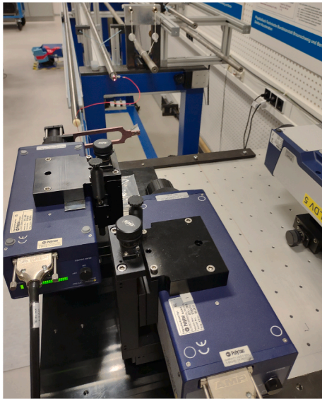
Fig. 1. LDV beams on the Hopkinson bar with a DUT.
