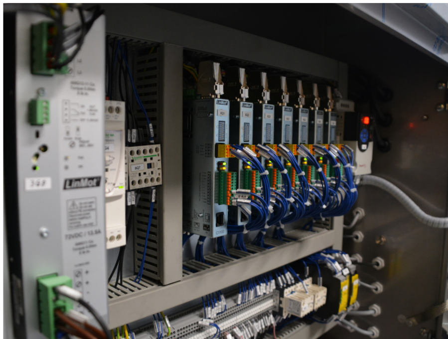
Optimal application for linear motors: servocontrollers with integrated safety, and power supply modules from LinMot.. (Photo: Rossmann)
