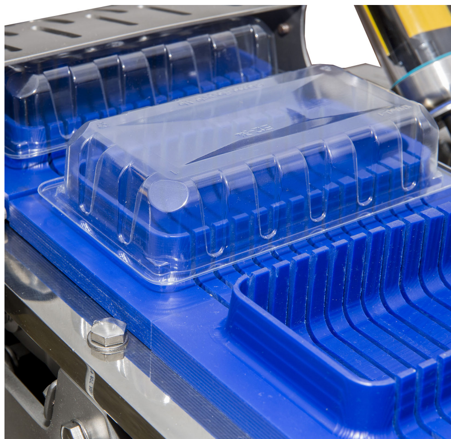
Product carrier with a recess in the shape of the product to be cut, to retain the original shape of the product. (Photo: Thielemann)
