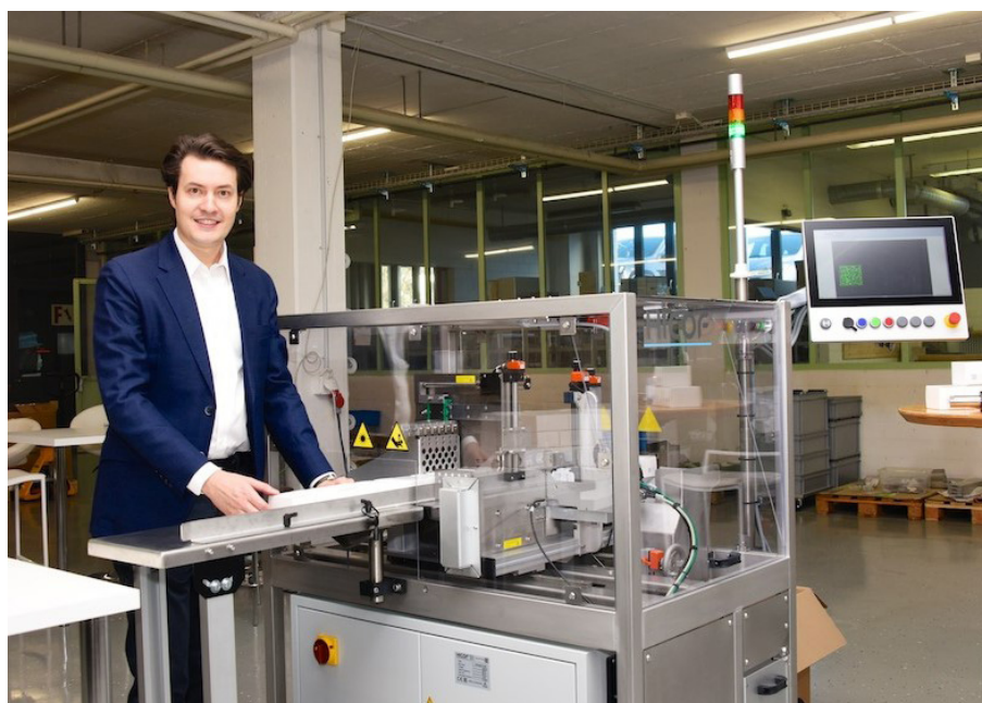
A flagship of the Hicof machine lineup, the AMACODER, aligns packages with millimeter precision. Without the repeatability of LinMot drives, this level of precision would not be possible.
