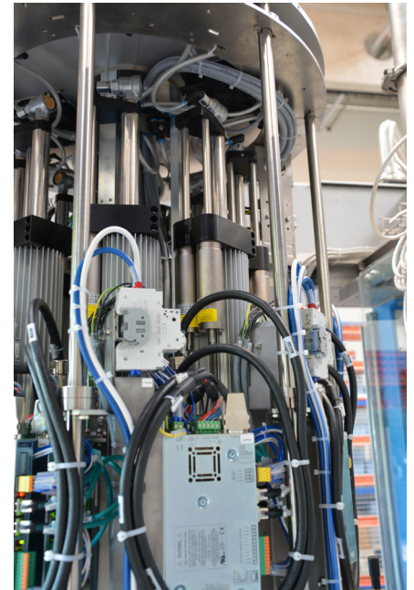
Magnetic springs (to the right of the black heat sink in the image) compensate for the weight of the closure spindle and maintain a safe position even when power has been disconnected.
