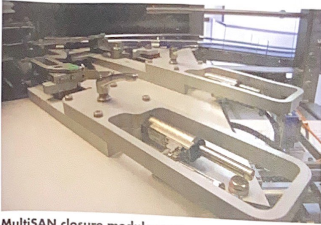
MultiSAN closure modules can be moved with a few manual steps to complete format change in minutes.
