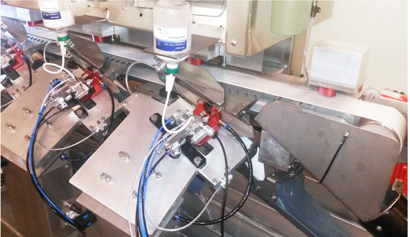
Based on the individually calculated injection depth and site, the LinMot linear motor precisely positions each vaccination station. (Photo: Rossmann)
