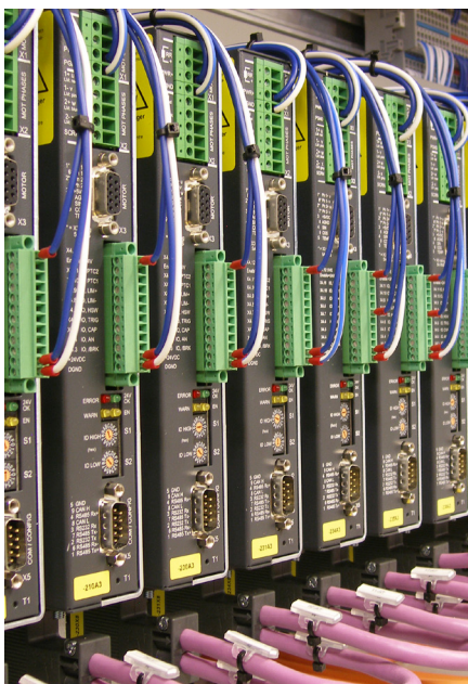
The linear and servomotors on the Z-110 are controlled by particularly compact servocontrollers from LinMot, with a PROFIBUS interface (DP) and 15A maximum current. (Photo: Zellwag)
