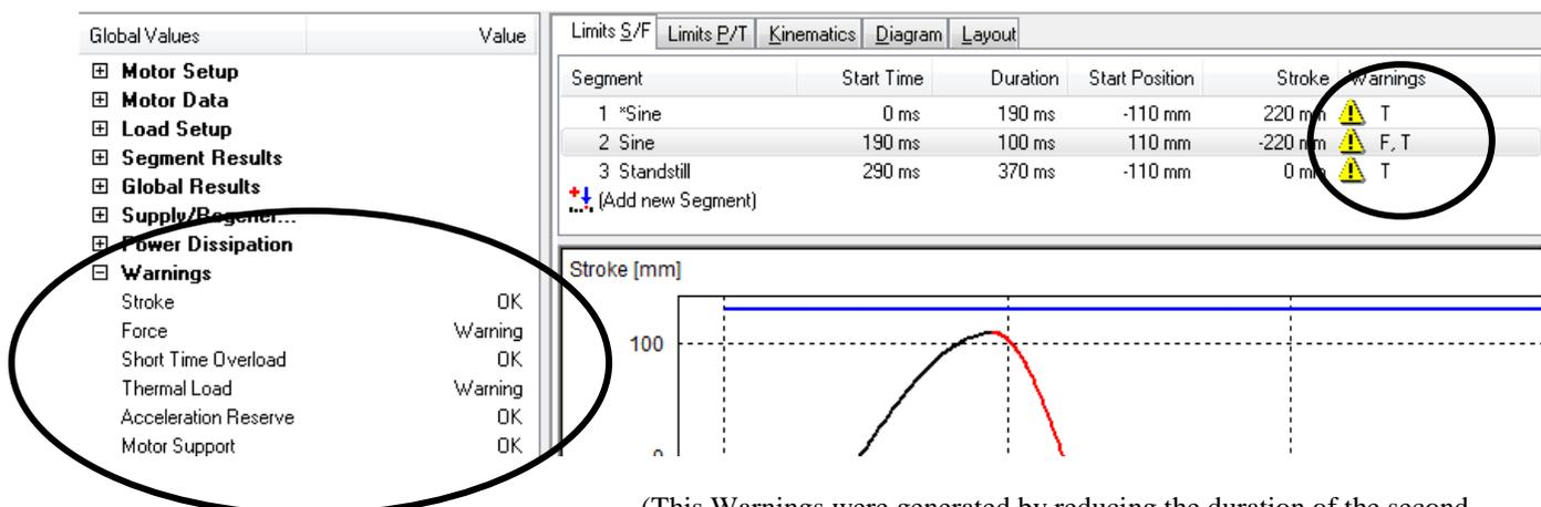
(This Warnings were generated by reducing the duration of the second segment in the example.)
