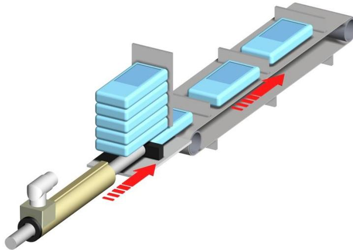
To handle the 82 products per minute, the minimal cycle time to push one product onto the conveyor belt is 730msec. In order to guarantee gentle product handling (and for dynamic reasons), a LinMot linear motor will replace the pneumatic cylinder.
