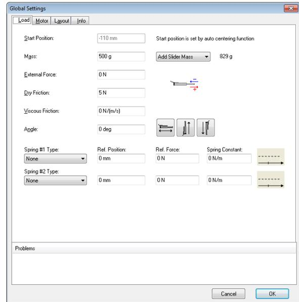
In the “Load” menu, the specification about the mechanical configuration (mounting, friction, zero Positions, etc.) has to be specified according to the construction.
