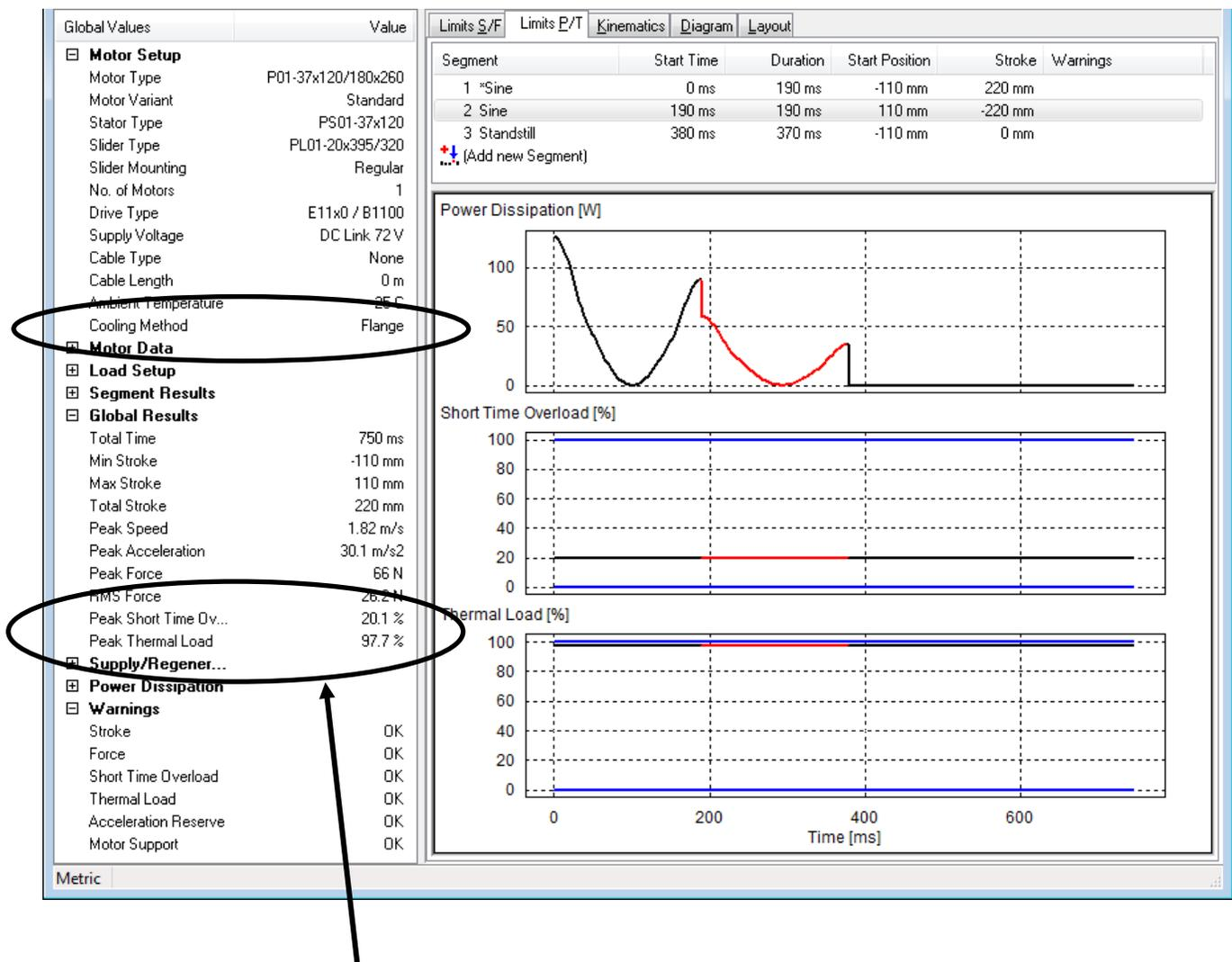
The Peak Short Time Overload Protection Value is definitely under the limit. The Peak Thermal Load is about equal to the limit, so the linear motor will not overheat in the application. If payload or friction will increase (or cycle time will be reduced), the Thermal Load will increase and exceed the limit. Then, the linear motor has to be mounted on a flange with fan cooling.
