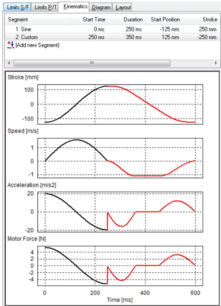
In “Tutorial\_Ex3.ldc” a Custom curve (Segment 2) follows on a Sine curve (Segment 1). The data vector of the custom curve was imported (loaded) from the csv-file “Tutorial\_Ex3.csv”. With a (negative) Scale value of -250%, the curve data points (forward motion from 0..100mm (in)) are scaled to a backward motion from 0..-250mm, starting at the end of Segment 1.
