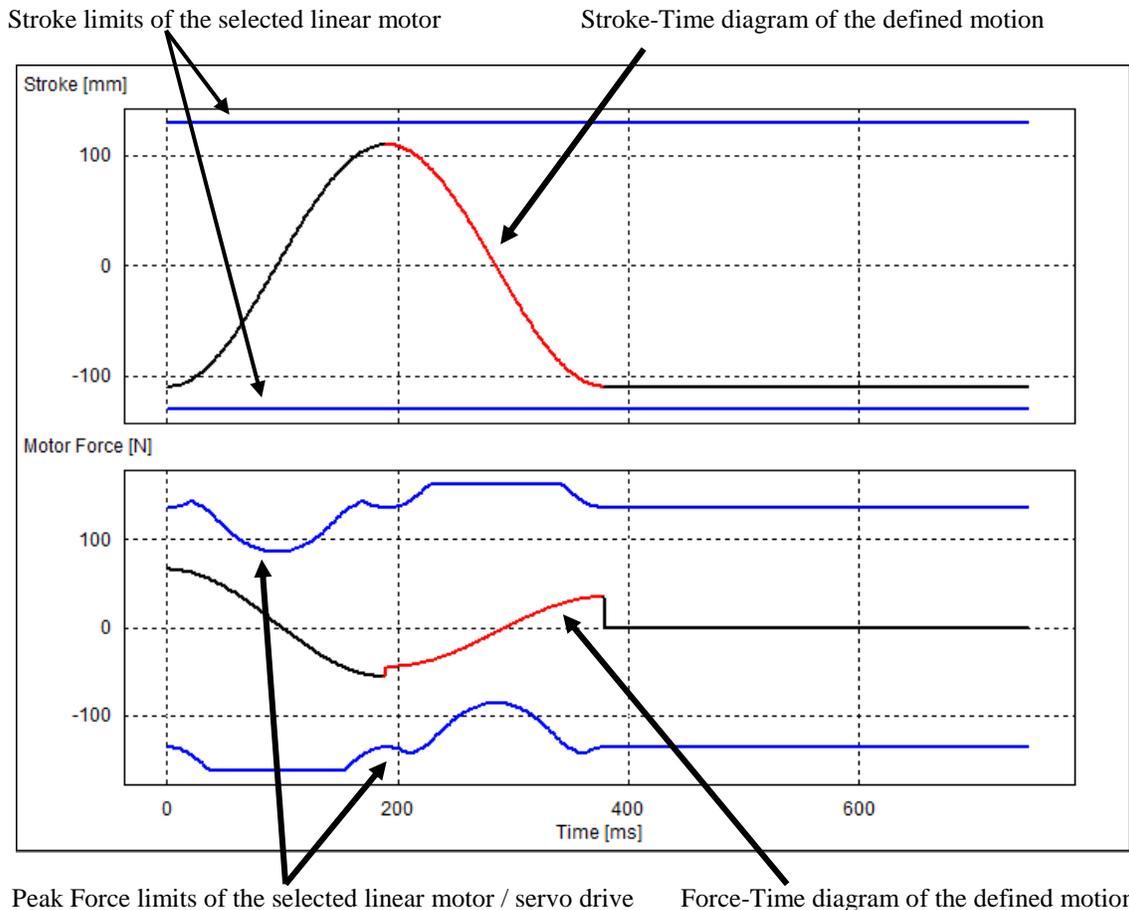
**Note:** Peak force limits of a linear motor depends on the actual position (see stroke force diagram in the data sheets) and on the actual velocity (peak force is decreasing with higher velocities). The peak force may change if another linear motor is selected due to differences in slider mass.
