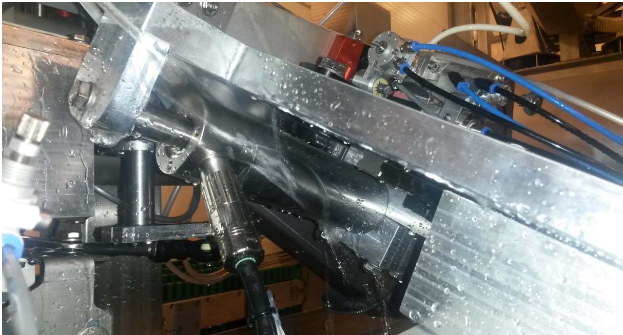
3: The especially compact stainless steel linear motors from LinMot used for positioning have a protection rating of IP69K, are absolutely watertight, and meet the most stringent hygiene regulations.
