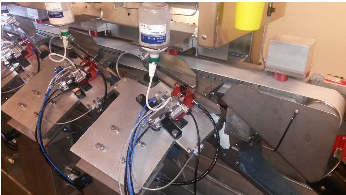
4: Based on the individually calculated injection depth and site, the LinMot linear motor precisely positions each vaccination station.
