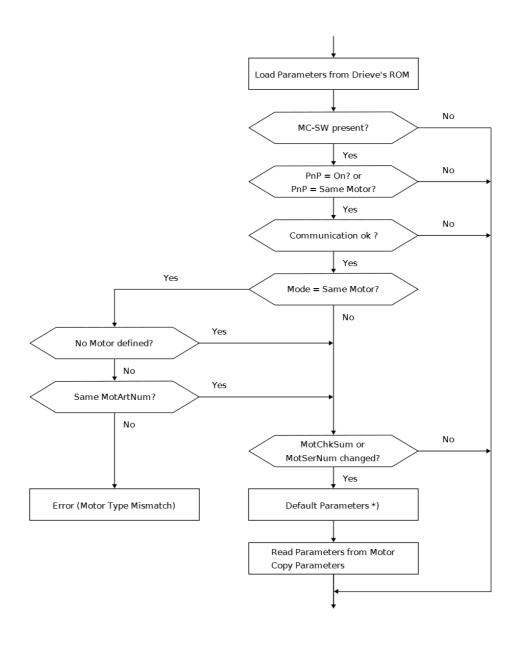
\*) All parameters, which are set by the previous PnP motor and do not exist in the new motor will be set to default values prior to load the new parameters.
