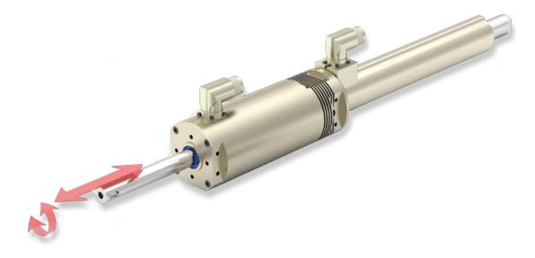
The PR01 motor series combines linear and rotary movements in a single integrated direct drive solution. The two motors are individually and independently driven. Working with a higher-level control high dynamic linear and rotary movements can be realized. These can be programmed either synchronously or independently of each other.
