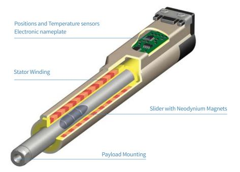
LinMot linear motors employ a direct electromagnetic principle. Electromagnetic force provides direct linear movement without the use of cams, gears, belts, or other mechanical devices. The engine consists of only two parts: The slider and the stator. The slider is made of neodymium magnets in a high precision stainless steel tube. In the stator are the motor windings, the bearing for the slider, the position detection and temperature sensors for thermal monitoring of the motor.
