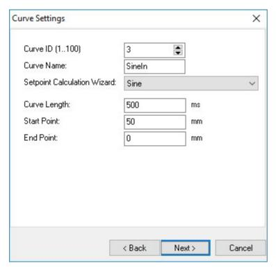
Set curve ID to 3, Curve Name to "SineIn", Curve Length to 500ms, Start Point to 50mm and End Point to 0mm. Click twice "Next" and then "Finish". Now we have defined the two curve segments and will join them together. Select the two curves
