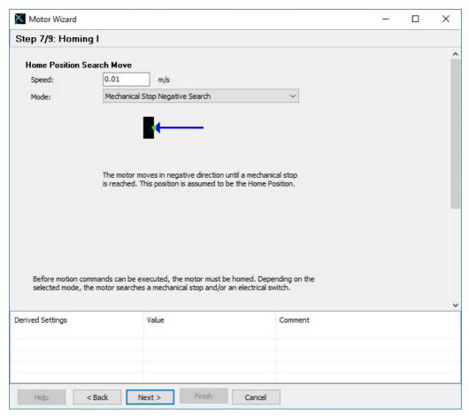
The most frequently used homing mode is "Mechanical Stop Negative Search". In this case the slider will move with the notch towards the stator's front end (where no cable is).
